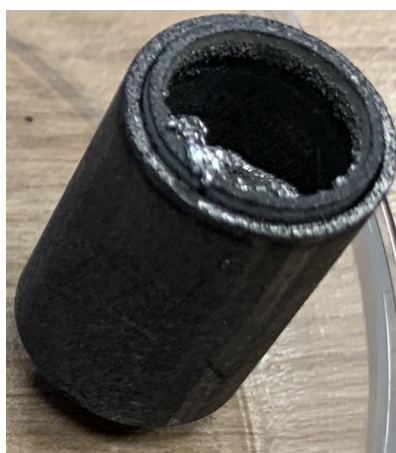
Example 2: Sample which migrates to the upper electrode
