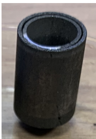
Example 1: Tin layer on the crucible
